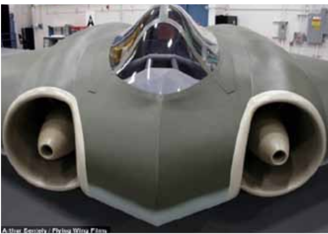
This full-scale replica of the Ho 2-29 bomber was made with materials available in the 40s
